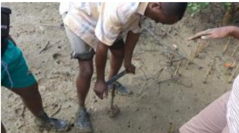
Figure 45. The sampler is now properly driven into the sediment and can be turned around by the handle until it moves easily
