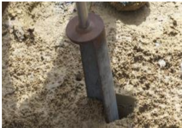
Figure 44. The sampler has been driven down in a tilted position, not in the proper vertical position. Tilting will probably result in a disturbed core that has to be discarded. Furthermore, the sampler is not taking the optimal sediment core because it is still too high.
