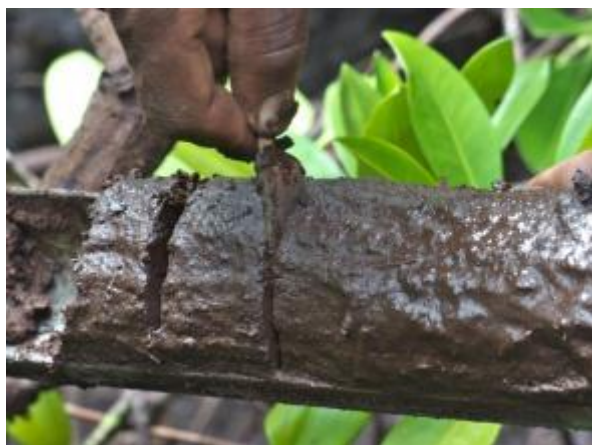
Figure 49. The excess bottom part of the sample has been removed and the subsample is cut to perfection using a sharp knife.
