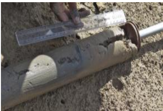
Figure 46. Material is missing from the upper end of the core. It may still be possible to extract the 0-15 cm slice. The crack in the core may not mean lost sediment and discarding of the core. Inspect the crack walls for corresponding features on both sides.
